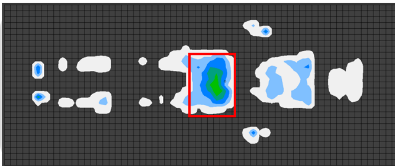
No support. Pressure readings: Heel= 55mmHg, Bottom= 69mmHg, Average= 33mmHg.
